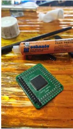
2. Place the syscon on the board (only the desired pinout)
